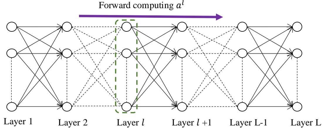
$$a^l = \begin{bmatrix} a_1^l \\ \dots \\ a_j^l \\ \dots \\ a_{n_l}^l \end{bmatrix}$$
