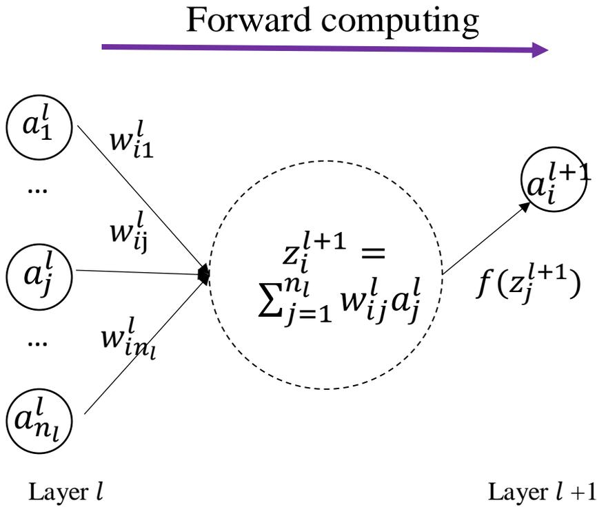
Component form  $\left\{ \begin{array}{l} a_i^{l+1} = f(z_i^{l+1}) \\ z_i^{l+1} = \sum_{j=1}^{n_l} w_{ij}^l a_j^l \end{array} \right.$
