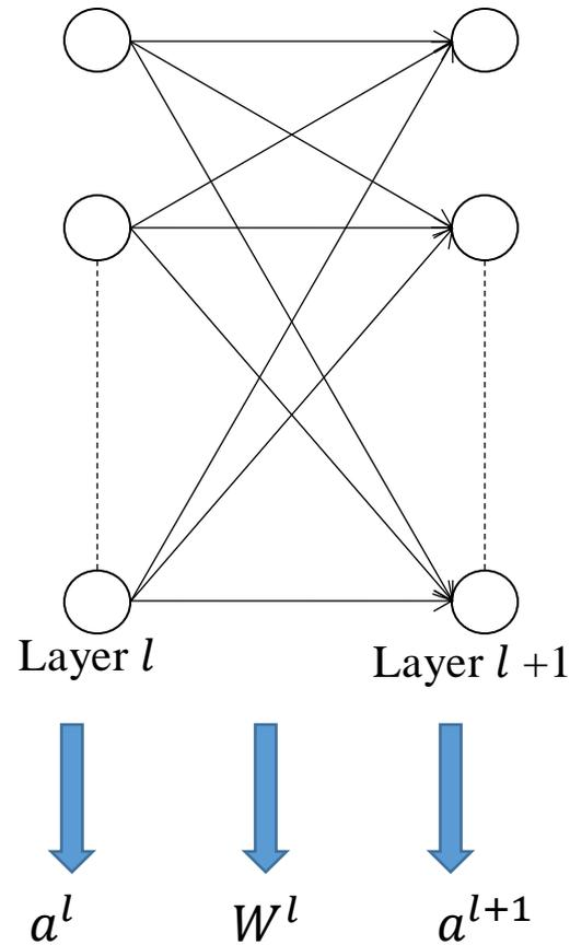
Vector form  $\left\{ \begin{array}{l} a^{l+1} = f(z^{l+1}) \\ z^{l+1} = W^l a^l \end{array} \right.$
