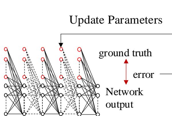
**Supervised Learning:** Update the network parameters according to the error between the target output and the actual network output of the training sample
